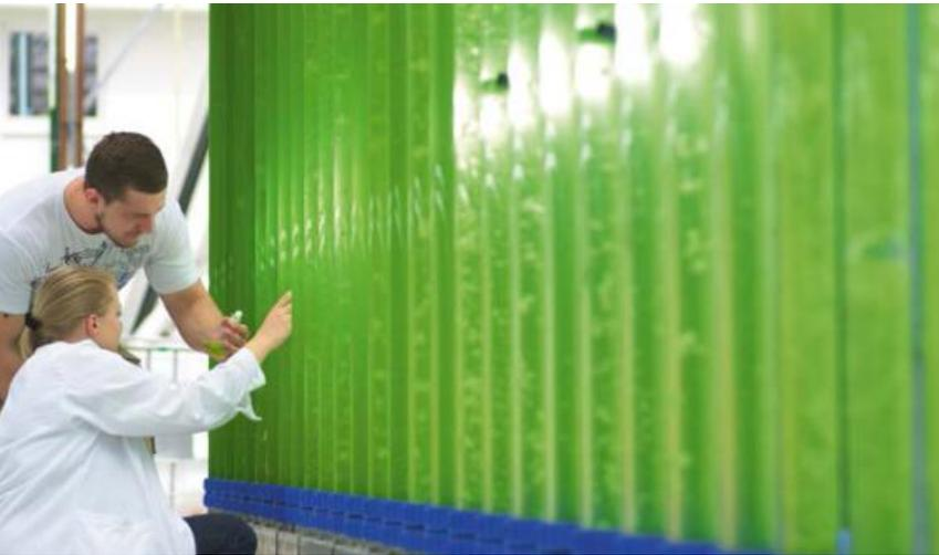
**By using high-quality, round DURAN® glass tubing from SCHOTT, the light that algae need for photosynthesis can be put to better use in photobioreactors. Tubes and multiple distributors are also ideally suited for constructing state-of-the-art vertical photobioreactors.**
